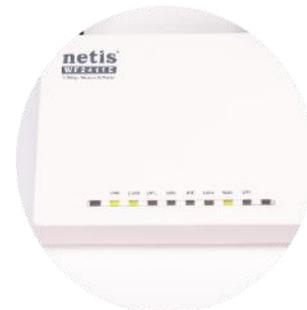
Plug the LAN cable into the BLUE 'WAN' socket on the the Netis router. Plug the other end of the LAN cable into the internet source (your internet router or Network socket)
