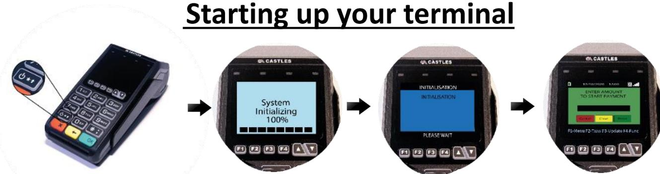
Press and hold the power button (above the red key) until the screen lights up. The terminal will power on and initialise for use
